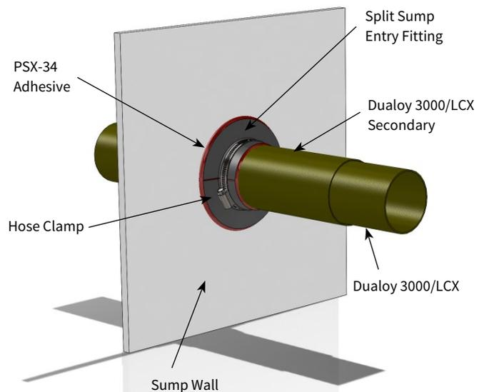
Complete Split Sump Entry Fitting assembly example
